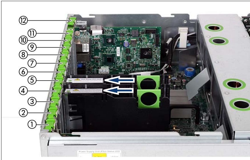
Figure 22: PCI slots with and without hot-plug functionality
